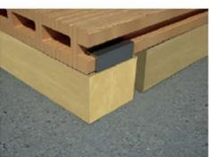
The starter clip can be used as a finishing clip. Install the clip to the end of the last joist, slide the deck board between the last clip and the starter/finishing clip
