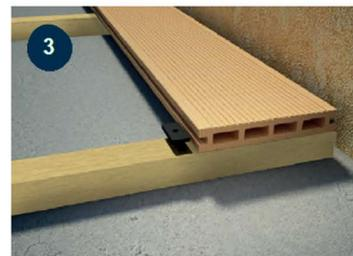
Slide the deck clip into position along the bearer (joist) until it is located against the deck board.
